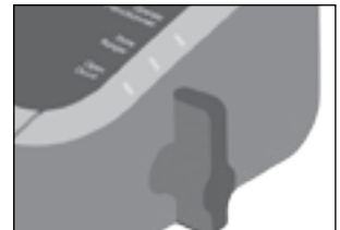
Push the latch into the center position to store.
