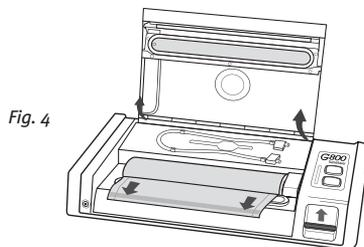
5. Pull out desired bag length, Close Appliance Lid, and slide Bag Cutter across the roll. Make sure you leave 3” of space at top for room to vacuum seal. (Fig.5)
