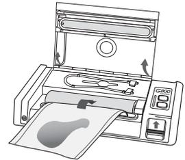
4. Close the Lid by pushing latch all the way down past the Store Position to the Closed Position. (Fig. 3)
