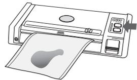
6. When the Red Indicator Light turns off, unlatch, lift lid, and remove bag. (Fig. 5)
