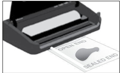
Place Bag in Vacuum Channel
