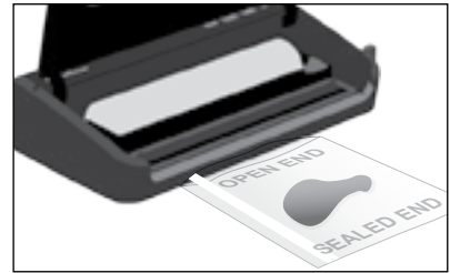
Place Bag on Sealing Strip
